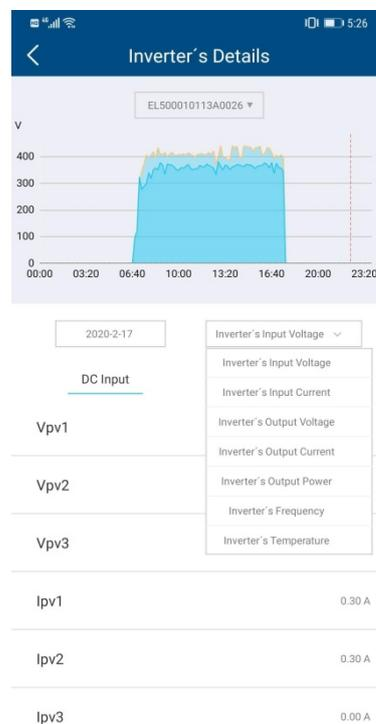
Figure 2-4-1-6 Curve switching
